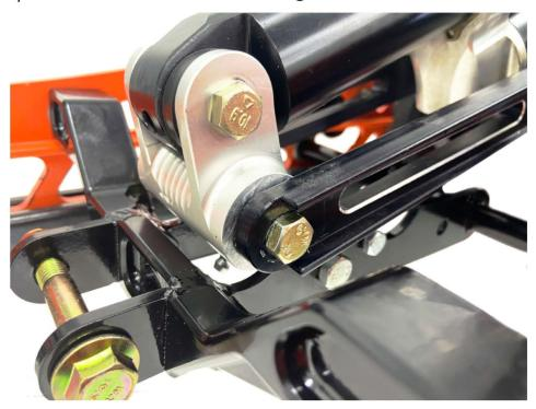
The bracket is needed to provide additional clearance for the cam pivot.
