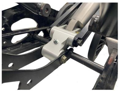
With a factory length shock the linkage will over cam when the suspension is not installed into the chassis.
