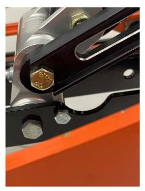
Movement can be restricted by installing a temporary stop (over cam bolt) This bolt needs to be removed once the suspension is installed or damage can occur.
