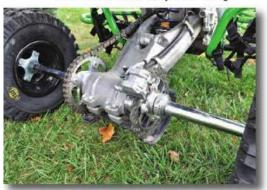
To widen our rear end for better cornering we installed a Durablue axle. Douglas Wheel Technologies Rokout front wheels and G2 rear wheels mounted with their MFX and MFR tires definitely improved tire and wheel durability and handling.
