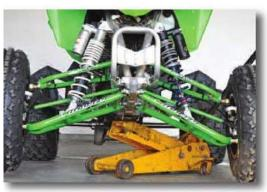
Notice the wheel travel difference between the stock shock on the left, and the Hygear shock on the right. Which would you rather have in the rough stuff?
