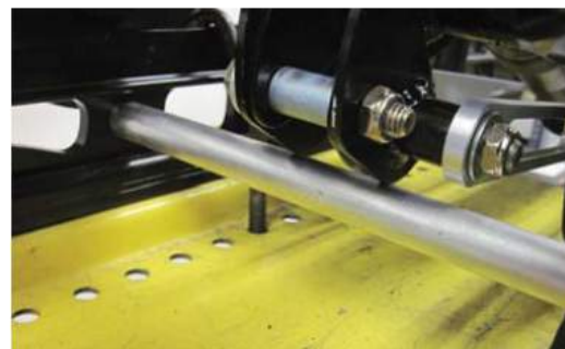
*Photo showing contact between the arm and the rear cross shaft before moving backward
