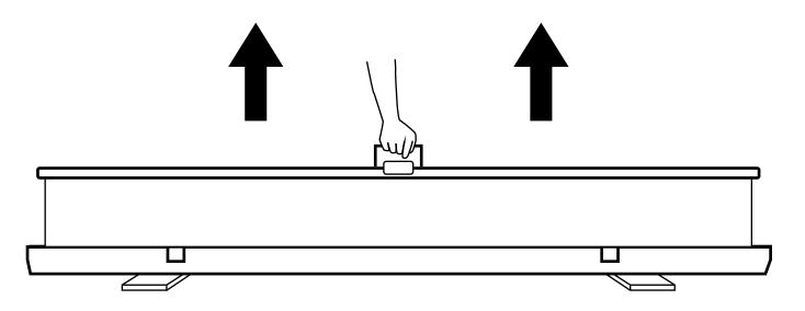
4. To extend the screen from the container, slowly pull out the screen at a perpendicular angle using the handle.
