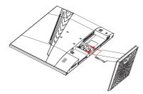
3 Insert the completed stand into the back of the monitor as shown in the illustration.
