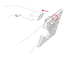
3 Lift up the small bar underneath the stand stem slightly, and then pull out the stand stem from the stand base.
