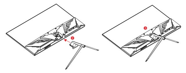
2 Take out the product with foam still attached, and gently place it on a desktop or table. And insert the stand stem into the back of the monitor as shown in the illustration.
