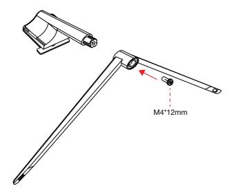
Open the package, assemble the stand base to the stand stem with 1 piece of M4\*12mm. Screw as shown in the illustration.
