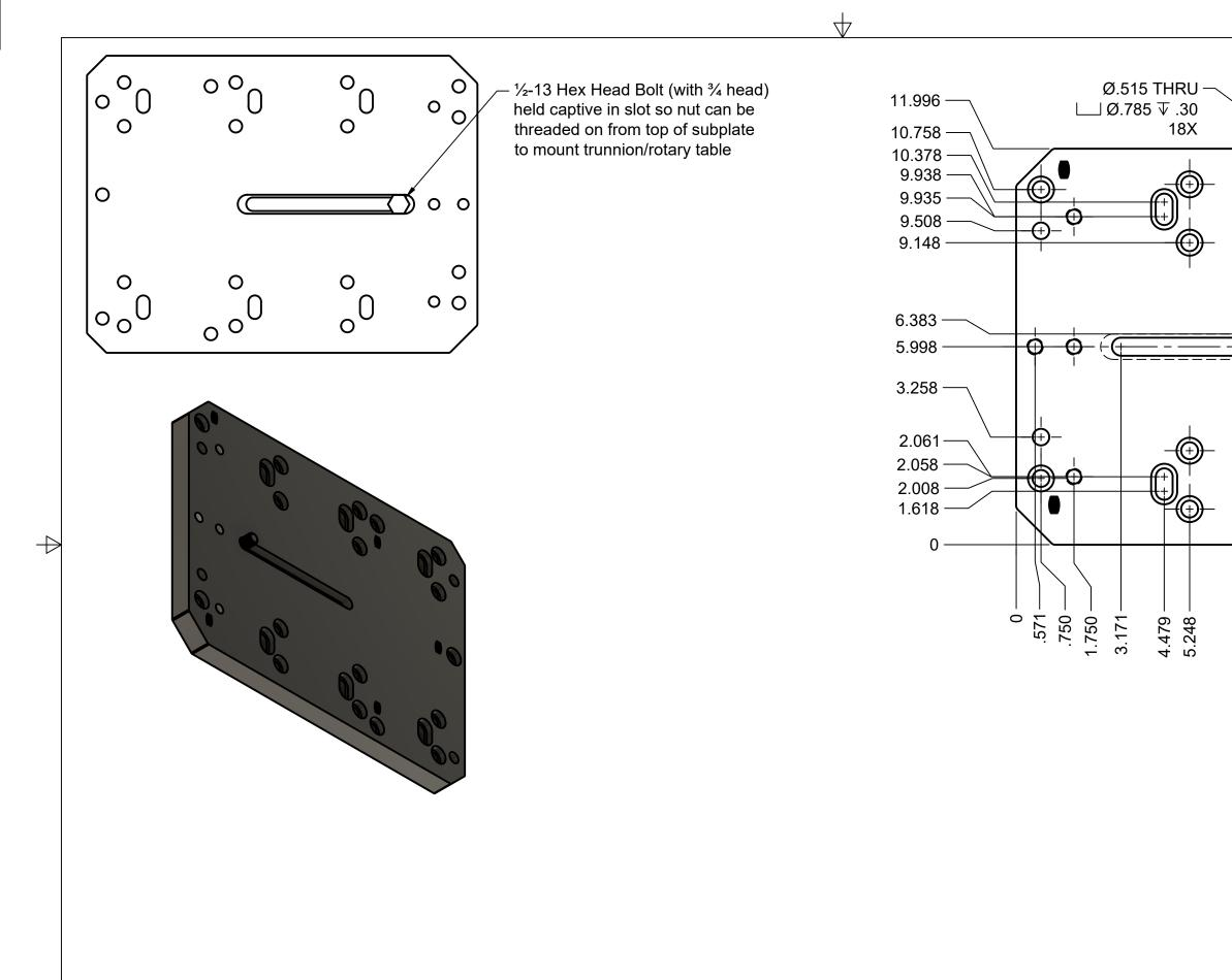
ADDITIONAL 1/2-13" THREADED HOLES MAY BE ADDED FOR USE IN THE MANUFACTURING PROCESS
