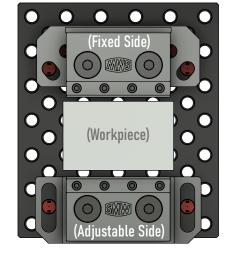
1. Place vise and workpiece on your fixture plate to determine hole placement. (Tip: use colored fixture plate plugs to mark repeat setups)
