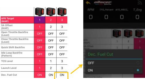
"ON" means no fuel injection when deceleration.
