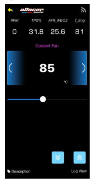
Coolant fan control. When the Engine temperature is over the threshold, ECU will turn on the fan. When the temperature is below 5°C of the setting value, fan will be turned off.
