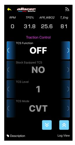
Traction control system is controlled by wheel speed or engine information. If TCS according to the wheel speed, when the rear wheel is sliding over the threshold, ECU will reduce the engine torque to control the percentage of slide and maintain the maximum acceleration.
