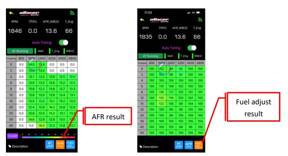
AutoTune processes full range internal fuel map correction to fit target AFR automatically with AF module (wideband AFR module).
