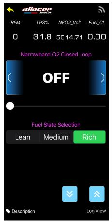
The function that corrects the fuel amount according to the signal of stock narrow band O2 sensor.
