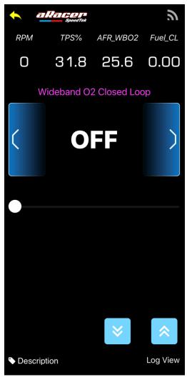
aRacer ECU can work with AF1/2 module (wideband AFR module) for wideband AFR closed loop. (WB O2 Closed loop corrects fuel amount more quickly than AutoTune, but the results will not memory in the ECU.
