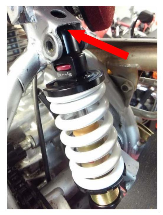
TBparts.com CRF100/XR100 shock was made to be as long as possible while getting the most travel out of the limited area available for the shock on these bikes. This makes for a tight fit and to install the shock, the top must go up into the top shock mount first (but do not bolt it in until you have bolted the bottom in).
