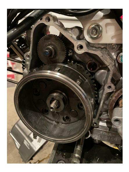
3. Remove oil pump on clutch side
