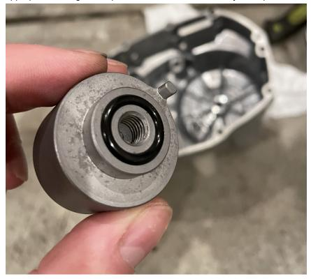
Tang on slave cylinder must be indexed inside marked recess inside clutch cover.
