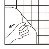
Remove film-face and remove excess thin-set from grout joints with a razor knife if necessary.
