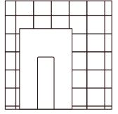
Lightly tap sheets with rubber grout float.
