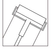
Apply a crack insulation membrane over substrate per the membrane manufacturer's instructions.
