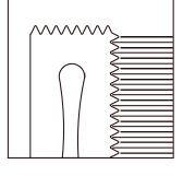
Use a V-notch trowel to apply a white glass tile thin-set mortar.
