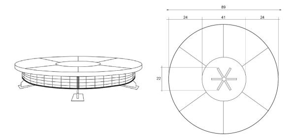
Note: Enclosure should be located a minimum of 3-4ft. away from fire feature. Ensure the enclosure is not placed directly on/over the propane hose that could otherwise kink, pinch, or cut off the gas supply.
