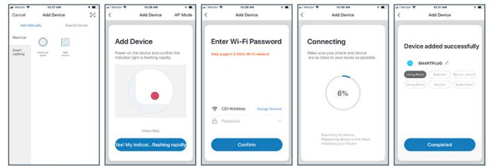
Follow prompts on app to confirm light is blinking and input wifi password. A window will show confirming the device has been added.
