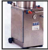
Equipped with wheels, pressure gauges, and waterproof electric switchboards.
