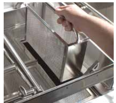
Built-in Scrap Basket for ease of cleaning
