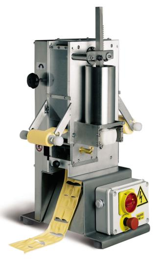
The Italiana FoodTech Ravioli Maker is available in both a manual, or automatic version. On the manual machine, the dough is fed through the machine with a hand crank, the automatic version does it all with the push of a button. With seven high quality ravioli molds to choose from, these ravioli makers produce pasta in a selection of different sizes and shapes to suit your needs and tastes.
