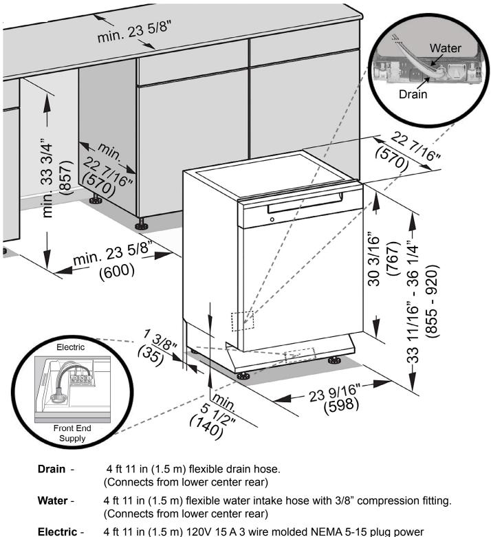
supply. (Connects via Front End Supply or may be hardwired)
