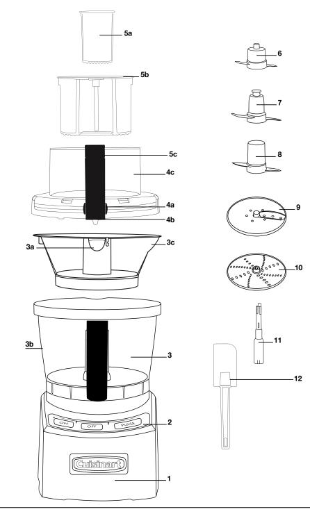
Note: The chopping/mixing blades should not be removed with liquid contents above the hub of the blade in the bowls, as this will defeat the SealTight™ system.
