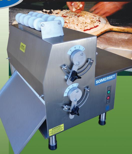
The veteran of side operated compact dough rollers. Sheets up to 20" (51cm) in diameter in seconds.
