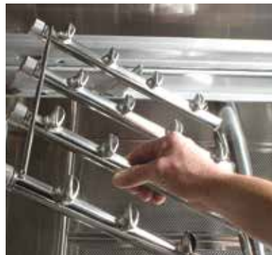
One-Piece Cast Stainless Steel Spray Assembly
