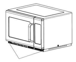
To re-install, align the filter to the holes and turn the screws right to tighten
