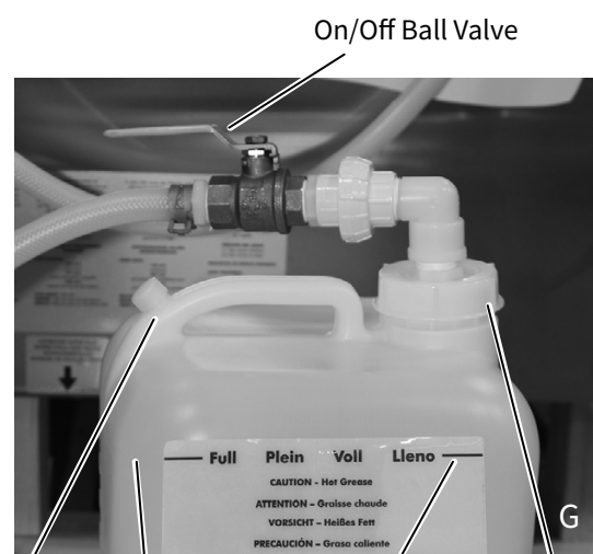
Vent Cap Grease Collection Container On/Off Ball Valve Recommended Capacity Container Fill Cap
