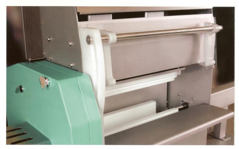
Easy loading of products into the mould when operator safety hatch is open and starting of slicing just by closing the hatch. "Cani it be simpler"!
