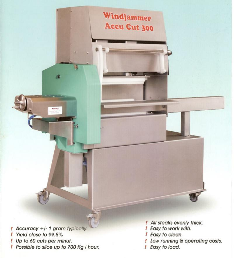
The Accu Cut 300 is designed to slice from fresh and slightly tempered boneless whole muscle meat into exact weight portions of Beef, Pork, Turkey, Liver, also tumbled and cooked. Generally all meat that can be formed can be sliced.
