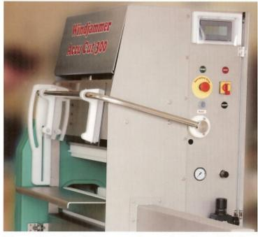
Operating touch screen panel and pushbuttons on right hand side of operator which makes them easy to access.
