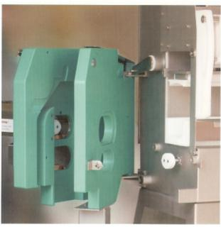
Extremely easy cleaning for excellent hygiene by opening the cutting chamber and removing the forming moulds. This is done in a few minutes.
