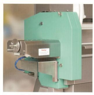
Easy adjustment of cut thickness / product weight by simply turning the handwheel. This eliminates the need for additional moulds for product weight thus saving in investment.
