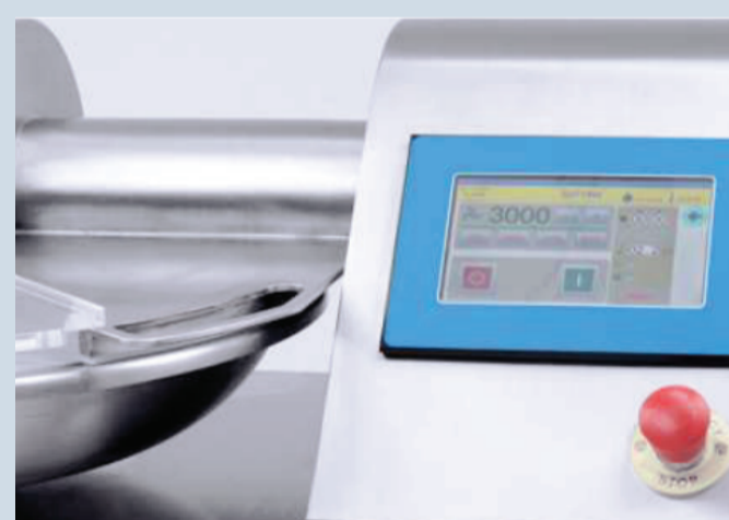
EMERGENCY STOP BUTTON
