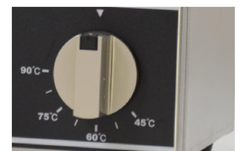
The temperature is controlled by an adjustable temperature dial which ranges from 45°-90°C.
