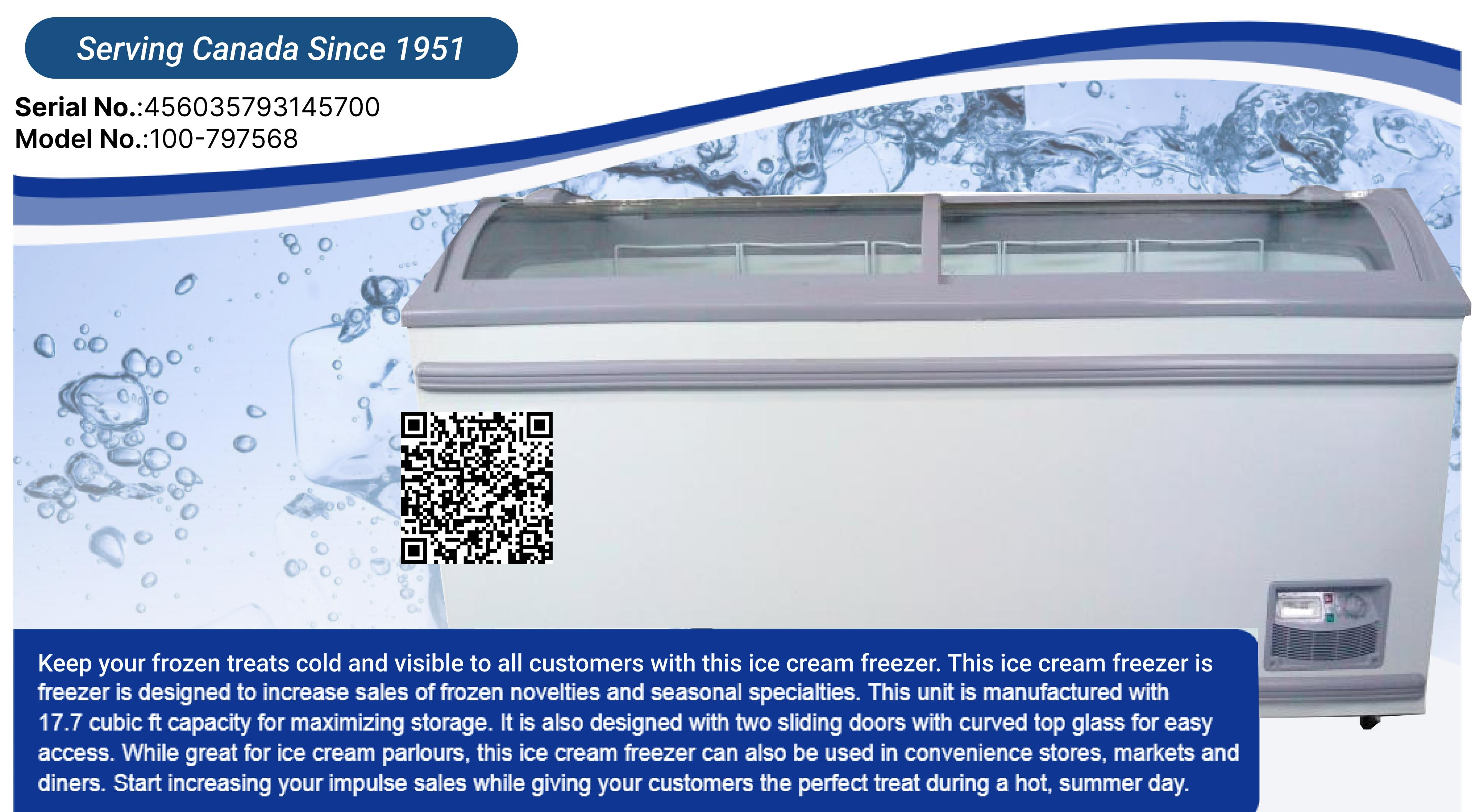
DESCRIPTION 17.7 cu. ft. ice-cream display freezer NET VOLUME 500 L / 17.7 cu. ft NUMBER OF DOOR NUMBER OF BASKET POWER 0.33 kW TEMPERATURE RANGE ≤-18°C / ≤-0.4°F ELECTRICAL 110 V / 60 Hz / 1 Ph REFRIGERANT R134a DIMENSIONS (DWH) 58" x 29.75" x 32.25" 1473 x 756 x 819 mm PACKAGING 60" x 31.75" x 34.75" DIMENSIONS (DWH) 1524 x 806.45 x 882.65 mm WEIGHT 80 kg / 176.25 lbs. PACKAGING WEIGHT 95 kg / 209.5 lbs. Item shipped on pallet
