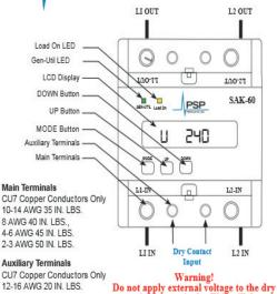
contact input terminals. This will damage the SAK-60 and void the warranty.
