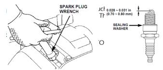
Clean and reset gap at .030" every 250 hours of operation. Do not blast clean spark plug. Clean by scraping or wire brushing and washing with a commercial solvent. Poor spark will occur if terminal does not fit firmly on spark plug. If this happens reform the terminal to fit firmly on spark plug tip.
