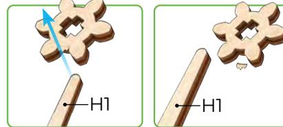
**ENG** Clean the burrs on the parts using the universal "Helper" (H) instrument.
