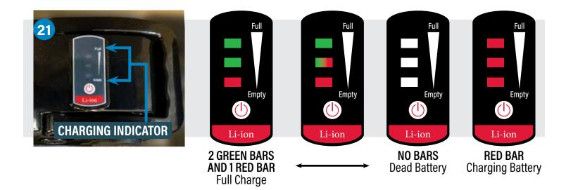
When the battery is finished charging, unplug the charger from the wall. **DO NOT** leave the battery connected to the charger unattended for an extended period of time.
