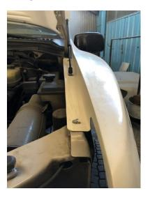
Once you have the fenders and hood mocked up they should be around 80% tightened up so there is still some movement for the fenders. Now you can bolt the bracket kit for the headlights and grill to the front of the core support so you can bolt headlights into each corner. \*\*you will have to rewire the new headlights to your older wiring\*\*
