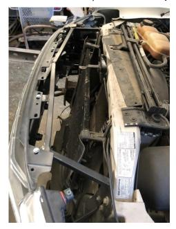
3) Once you have the headlights, hood and fenders attached and closely fitted about 80% you can now tighten up bolt up all parts for final fitment. Once you have everything fitted to your likings \*\* you will also have to relocate the hood latch release with a hood release extension to the lower section of the grill\*\*
