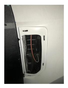
6) Head Light wiring form 99 to the new head light plug. Some head light models will very but for basic headlight that are halogen you should have 3 wires. GREEN/BLACK is hi-beam, RED/BLACK is low beam and BLACK is ground. The easiest way to convert headlights is to buy the pig tail plug in for the new 2017 headlights and splice into the factory truck wires.
