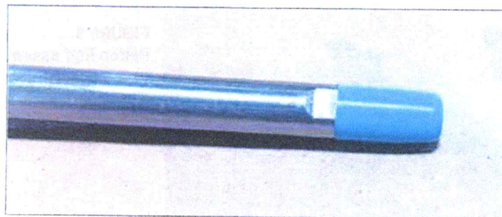
FIGURE 5 – PISTON ROD WITH INSTALLATION TOOL INSERTED
