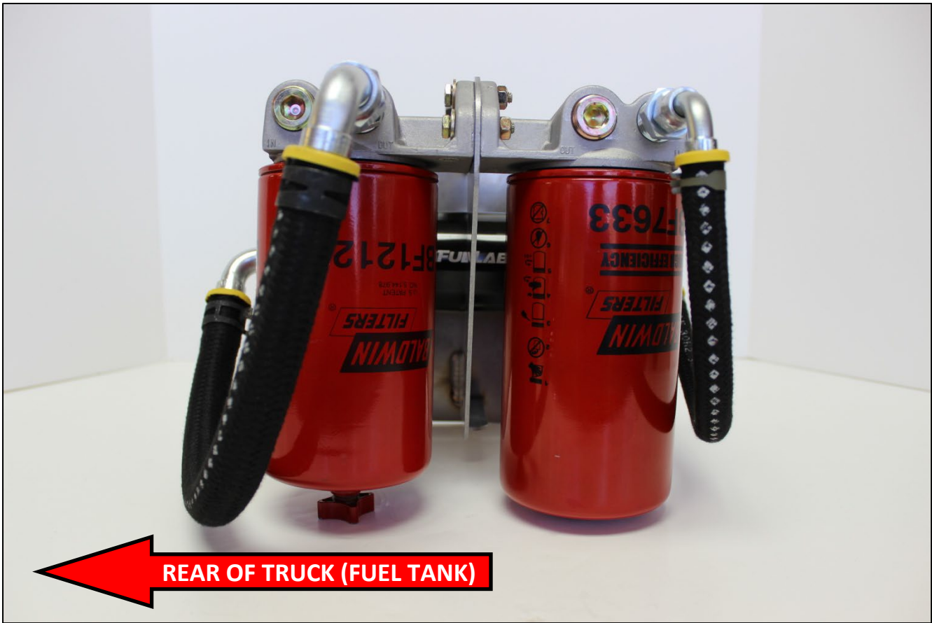
View from FILTER SIDE – Use this Picture for Hose Routing
