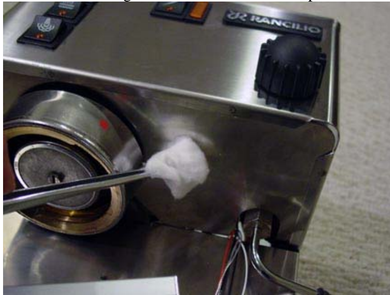
Figure 22. cleaning the box mounting area with alcohol.
