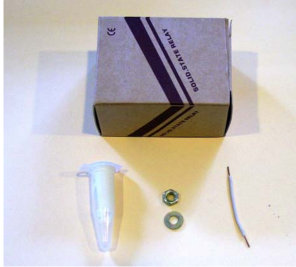
Figure 2. Solid State Relay (SSR), mounting screw nut and washer for SSR, silicone heat transfer compound (white paste in the vial) for SSR and sensor, and RTD jumper cable (see D 3)).
