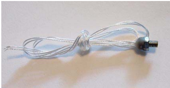
Figure 6, Temperature sensor (Pt100 RTD) with screw tip.
