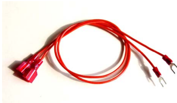
Figure 3, Cables for connecting SSR output to heater. Terminated with spade tongue terminal on one end and tab terminal on the on other end.
