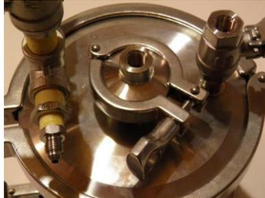
Figure 11: Attached tri clamp cap.
