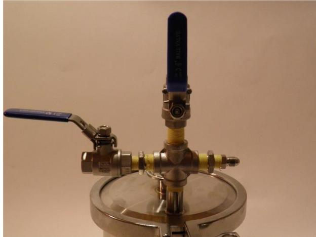
Figure 9: 3/8" Valve attached.
