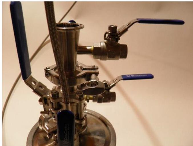
Figure 17: Concentric reducer attached to 3-Piece Ball Valve.
