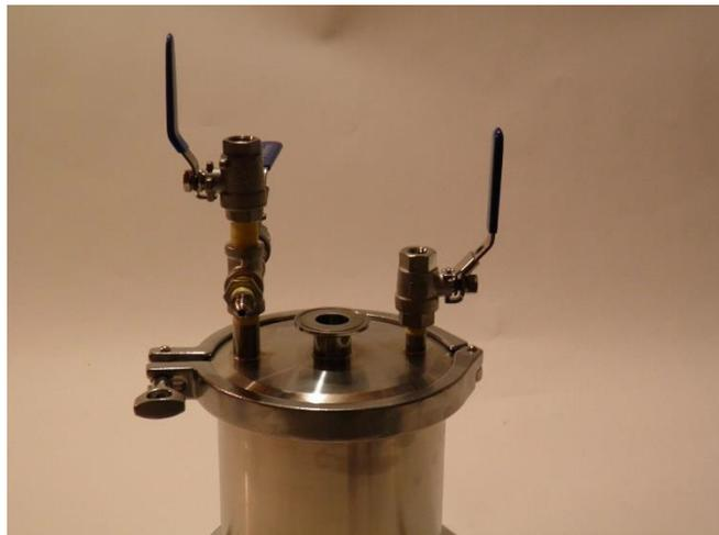
Figure 10: 1/4" Valve attached to lid.
