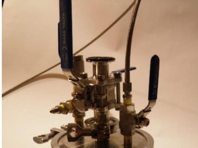
Figure 16: 3-Piece Ball Valve attached.
