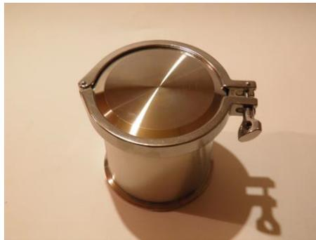
Figure 2: Collection pot with end cap installed
