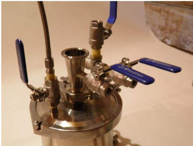
Figure 15: Concentric reducer with attached ¼" Valve
