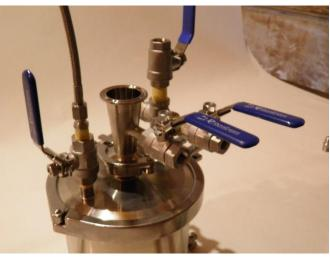
Figure 15: Concentric reducer with attached ¼" Valve
