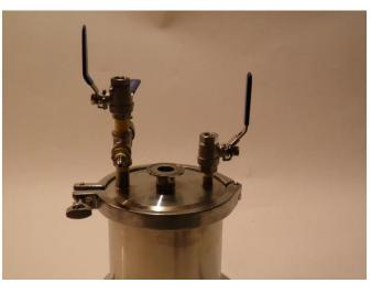
Figure 10: ¼" Valve attached to lid.
