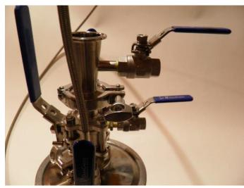
Figure 17: Concentric reducer attached to 3-Piece Ball Valve.
