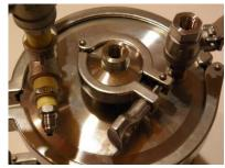
Figure 11: Attached tri clamp cap.
