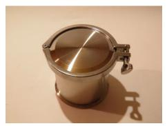
Figure 2: Collection pot with end cap installed
