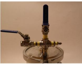
Figure 9: 3/8" Valve attached.
