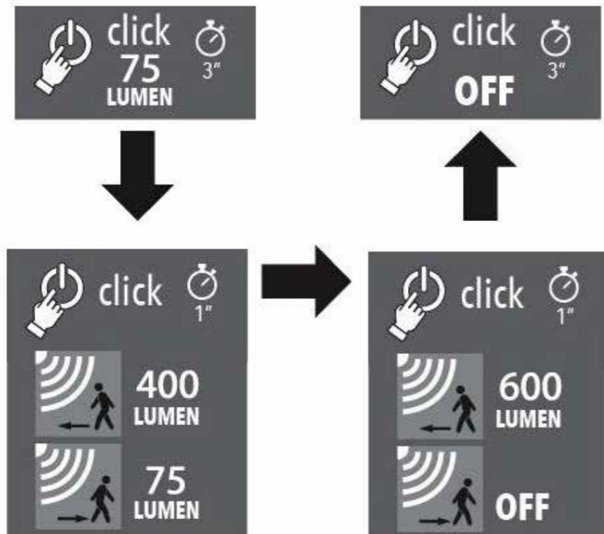
Click the button for 3s to light up the fixture, and it's mode A now; and then click the button for 1s, and it's mode B now; and then click the Botton for 1s, then it's mode C now; and then click 3s to off the fixture.
