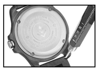
2) Depress the spring bar by applying pressure with the tool towards the watch band. When the spring bar is clear of the lug, that side of the band will drop down and out of the watch case.
