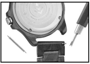
3) Rotate watch around and repeat these steps to the other side of the watch band. The watch is now ready for the leather replacement strap.
