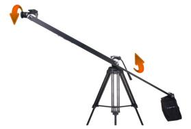
Tilting the camera relative to the Boom offers some interesting shots. Usually used in combination with other moves, Tilting can also be used on its own. Loosen the tilt drag on your tripod head. To tilt the camera, hold the weight bar in one hand and tilt the Pan/tilt handle on the tripod with the other hand. This allows you to change the tilt without changing the boom.
