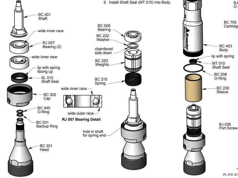
5. Insert Spring (BC 315) end into hole in Weights (BC 220), then slide Weights and Spring onto Shaft; insert other spring end into hole in Shaft.
