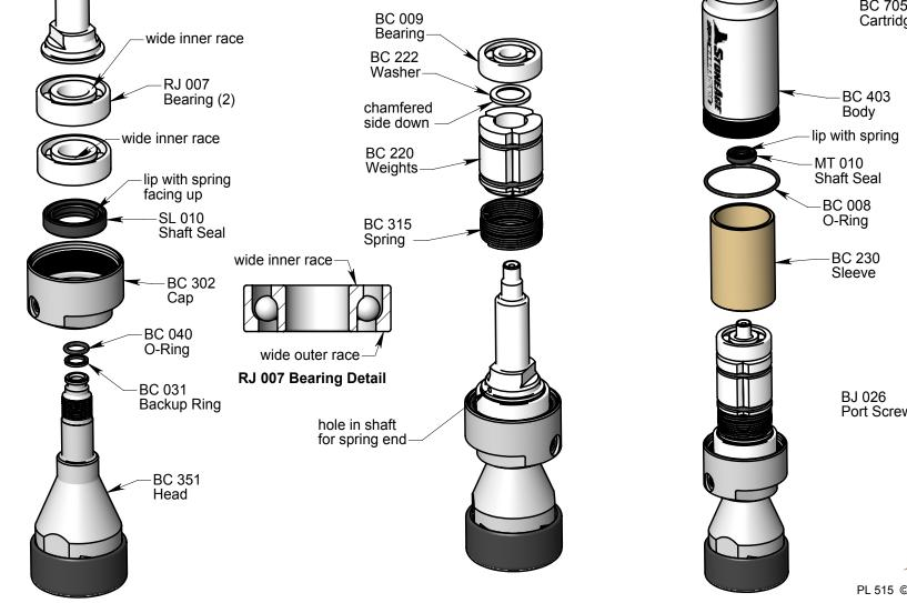
10. Apply anti-seize to threads of Body; thread into Cap. Tighten to 45 ft-lb.
