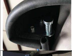
The striker is held with 2 M6 metric bolts, with allen heads on outside, and nylock nuts on the inside.
