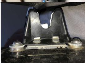
The latch is held by M6 metric button head bolts. The bolts are mounted into a bonded nut inside the camper, they can be loosened without anything dropping off. If a washer drops into the slot, it will fall out inside the rear hatch of the Element (eventually)
