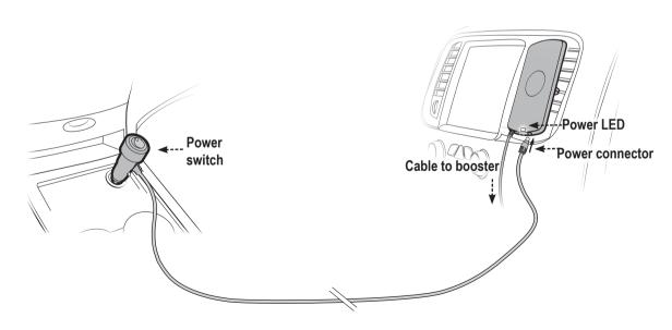
WARNING: The booster is rated for 5-15V input voltage. DO NOT use the booster with a higher voltage power supply. This can damage the booster and/or cause personal injury.
