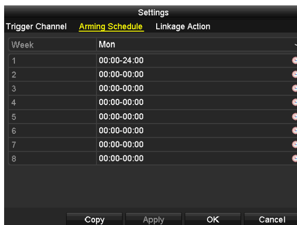
Figure 8.16 Set Arming Schedule of VCA Alarm
