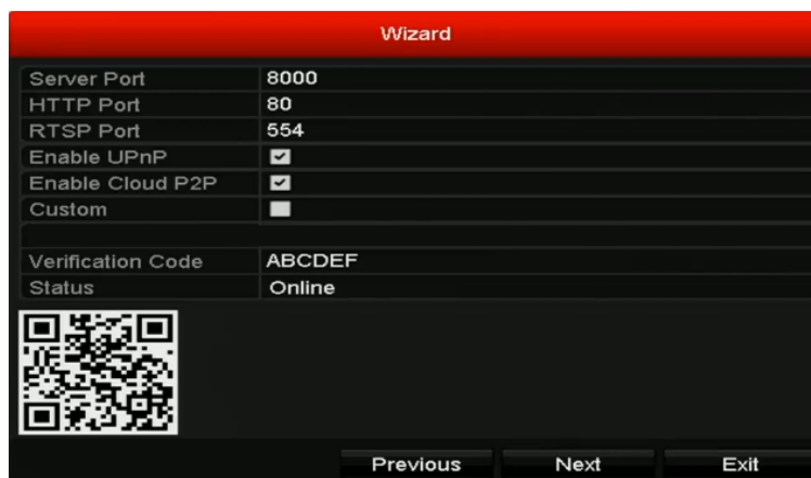
Figure 2. 8 Advanced Network Configuration
