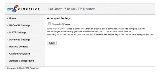
The B6000 has a timid DHCP server. This serves out an IP address of 192.168.88.90 to any machine connected to the router.
