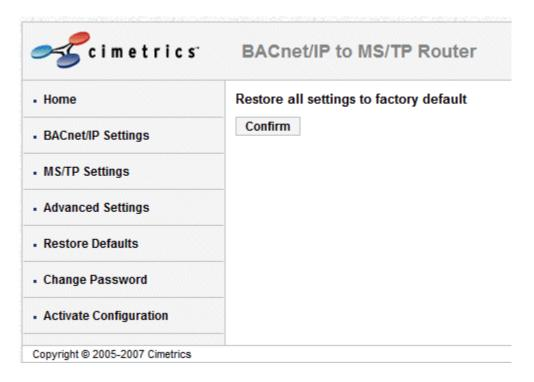
Clicking on "Confirm" will result in the ENTIRE configuration of the router being set to factory defaults.
