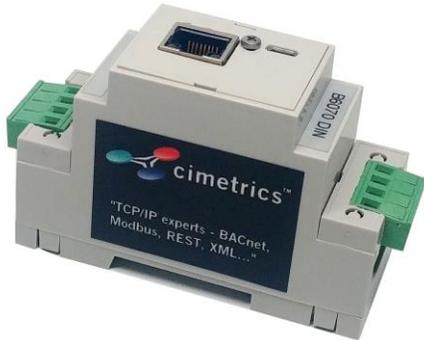
The idea of a pulse meter is to measure Consumption and Demand and timed or aggregated measures derived from these. Consumption is known by various names in various domains - energy usage in electricity, steam usage for steam, water usage for water. Demand is known by various names in various domains – average power in electricity, average flow for steam, average flow for water.
