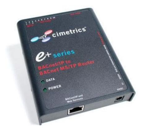
The Cimetrics B6000 is a BACnet/IP to BACnet/MSTP Router. It helps route BACnet communications from a BACnet/IP to BACnet/MSTP local area network, thus allowing BACnet/IP devices to communicate with BACnet devices on a BACnet/MSTP network. The Ethernet connection conforms to the BACnet/IP standard which is complemented by many network friendly features such as password protected browser based setup screens.
