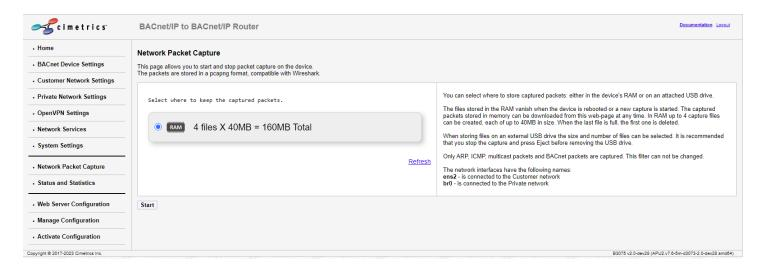
If you want to do a packet capture that is expected to require a considerable amount of memory, you can use a USB memory stick to store the files containing the captured packets. Insert a formatted memory stick into one of the B3075's USB ports, and then navigate to (or refresh) the Network Packet Capture web page. If the memory stick is recognized by the B3075, you should now see something like the following:
