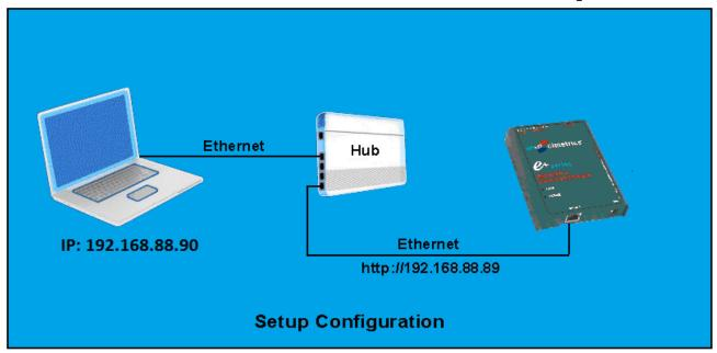
Access the B2000 configuration screen using your browser. Here is an explanation of how to do this:
